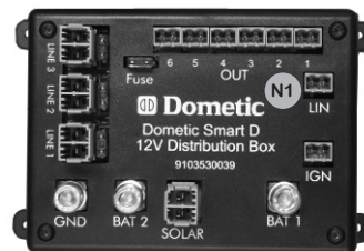
Elsystemets enhed N1. Dometic Smart D 12V Distribution Box.
